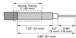
Fig. E RG8 Cable - Bottom Exit
